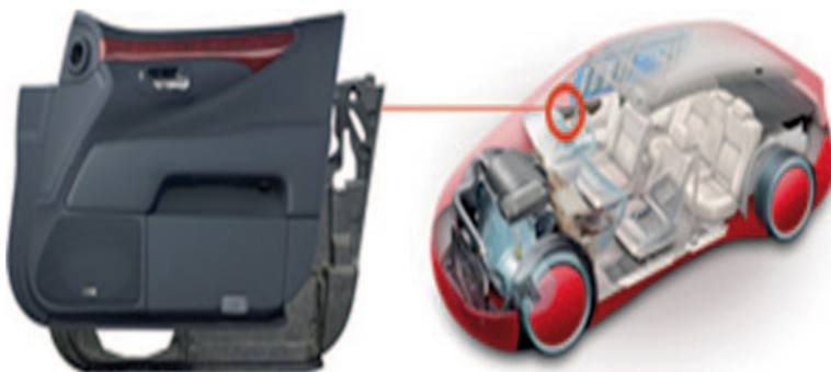
Fig. 11 The door trim using kenaf base material. (Source: Commercialization of door trims using kenaf and polypropylene (PP). http://www.toyota-boshoku.com/global/about/development/eco/kenaf/ )
