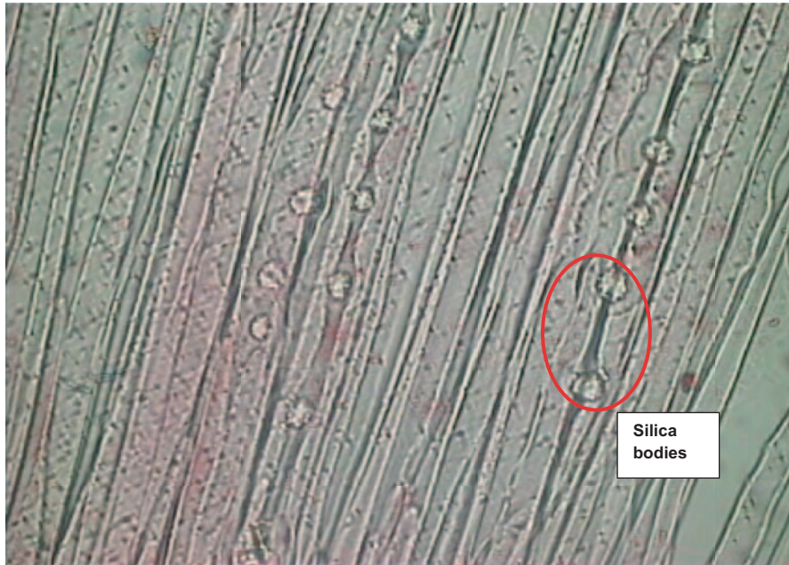
Fig. 3 Round spiky shape silica bodies found between fiber under microscopic magnification of 400×
