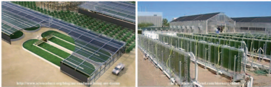
Fig. 8 Closed pond system and photobioreactor
