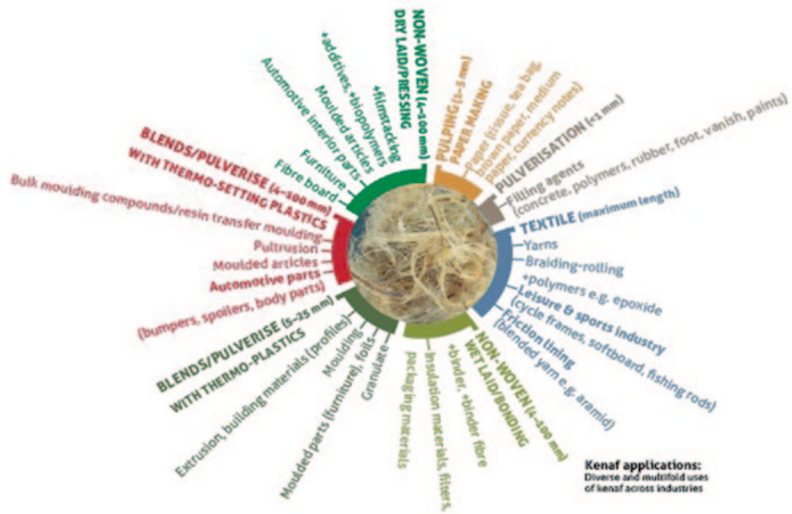
Fig. 6 Diverse and multiple uses of kenaf across industries (New Lightweight and Nanotechnology Enhanced Bio-composites from Lignocellulosic Materials, http://www.greenprospectsasia.com/content/fibrous-kenaf , Accessed on 24 June 2014)
